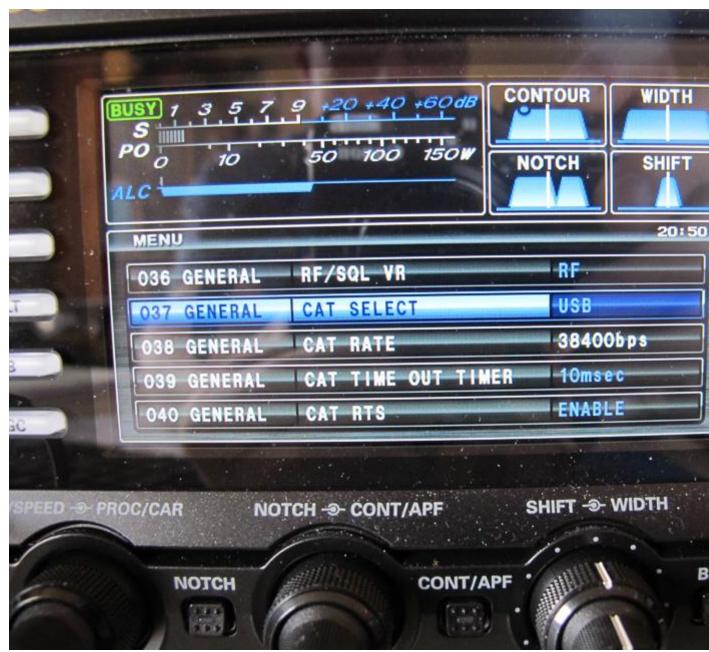
Menu settings applicable to the serial port When you setup HRD to connect to the radio ensure that the "Enhanced port" is being used and that the speed is the same as what was set in radio option #038.
